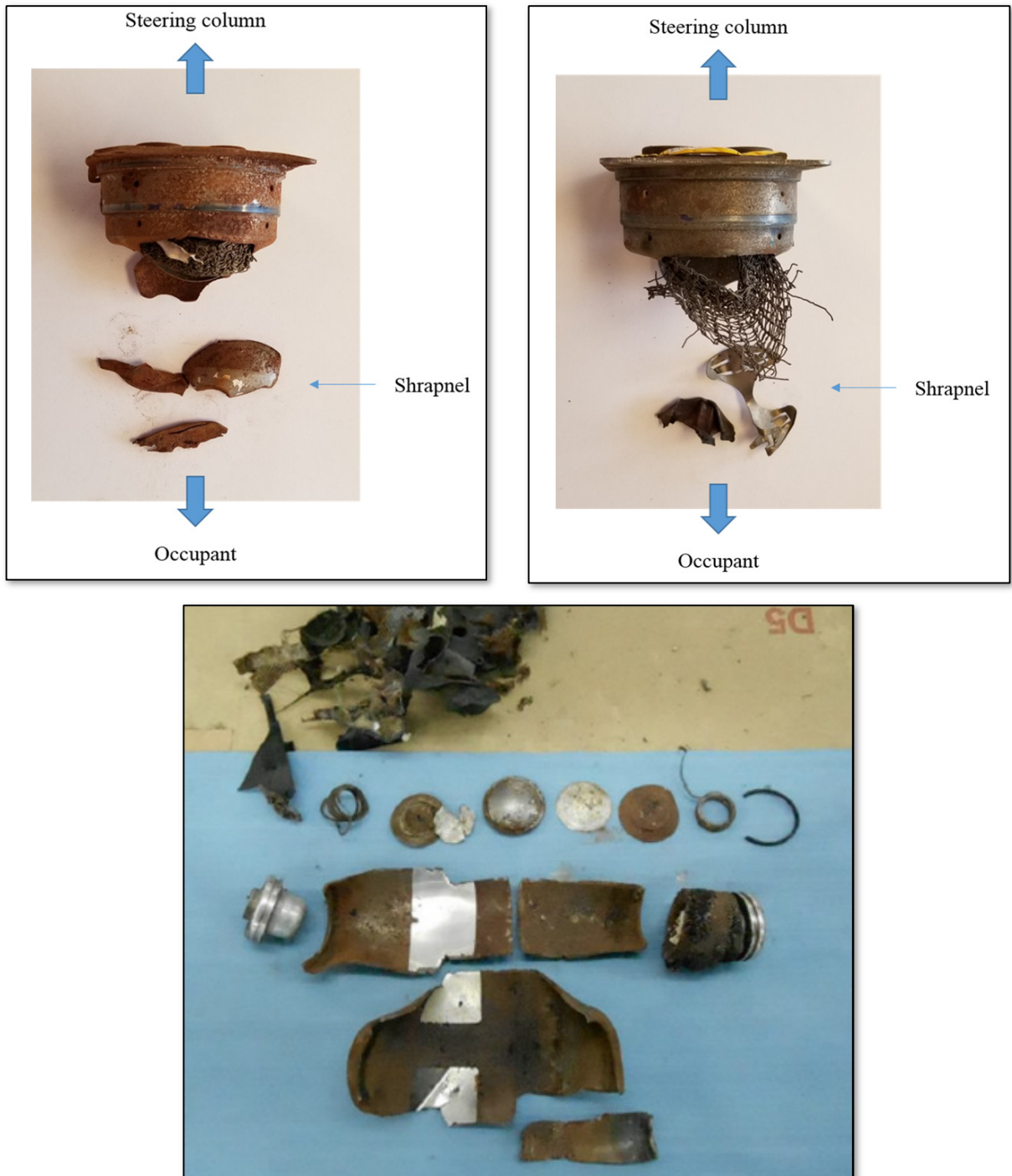
Figure 3: Photographs of Disintegrated Defective Takata Airbag Inflator Shrapnel Following Explosion
