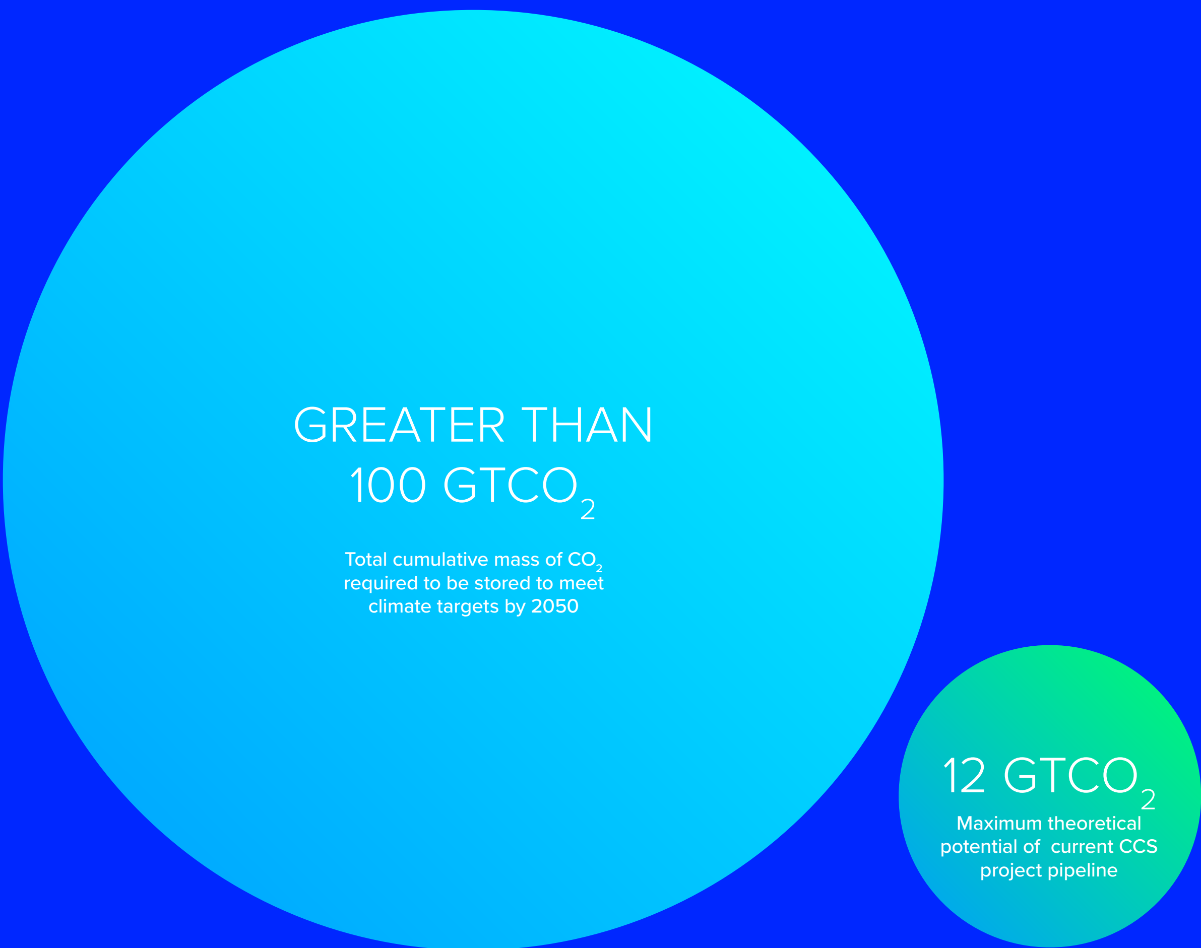
Figure 5.6–2: Comparison of total mass of CO 2 required to be stored by 2050 with the maximum theoretical potential of the current CCS project pipeline
