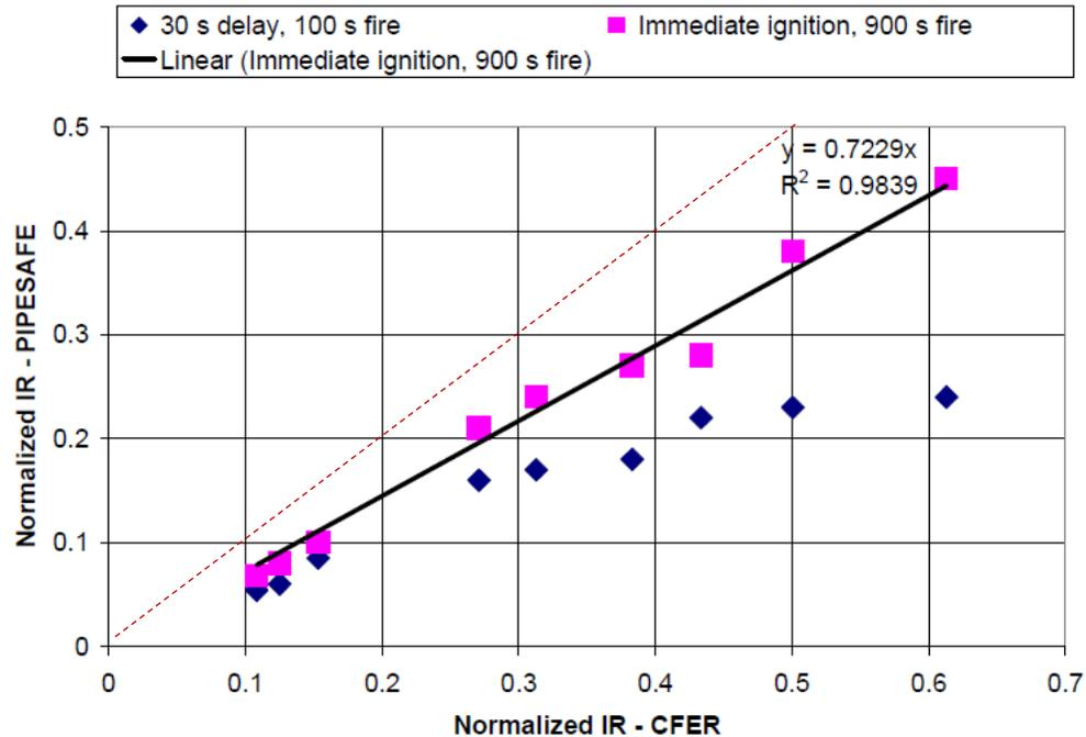
Results from C-FER model plot to the right of the unity line (i.e. dashed red line) indicating conservatism compared to PIPESAFE results
