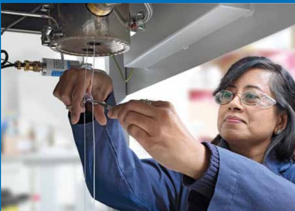
As part of our in-house testing, we use a capillary rheometer to evaluate the influence of Dynamar PPA on shear stress reduction.
