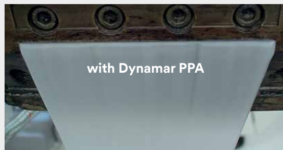
Reduction of die build-up in cast film extrusion
