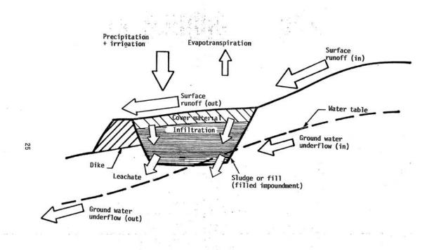
Figure 3-1. Simplified Water Balance for Filled Surface Impoundment
