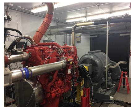
Heavy-duty engine test cell at EPA's National Vehicle and Fuel Emissions Laboratory. (EPA OIG photo)
