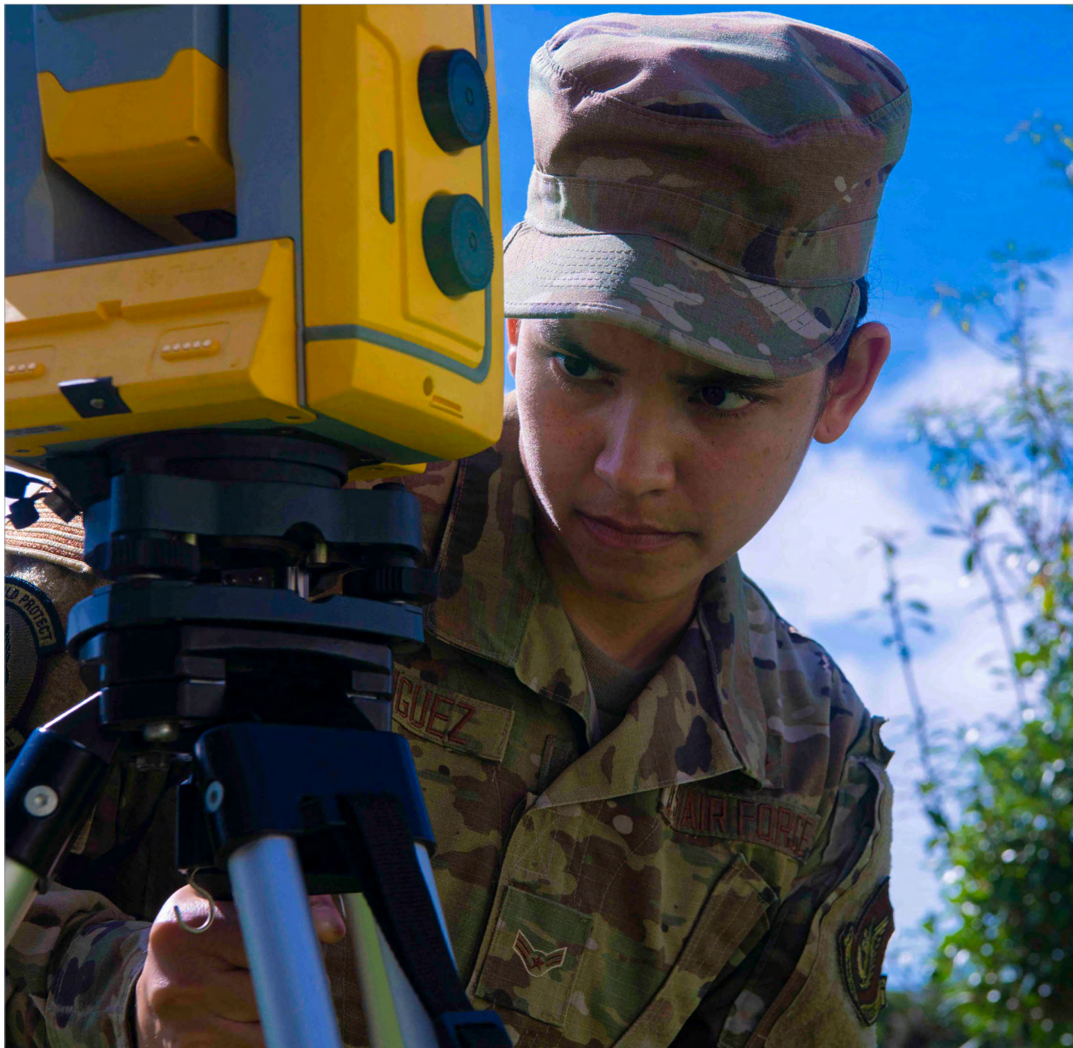
An Airman 1st Class, an engineering technician with 718th Civil Engineer Squadron, Execution Support, levels a Trimble S6 at Kadena Air Base, Japan, on June 9, 2021. (U.S. Air Force photo)
